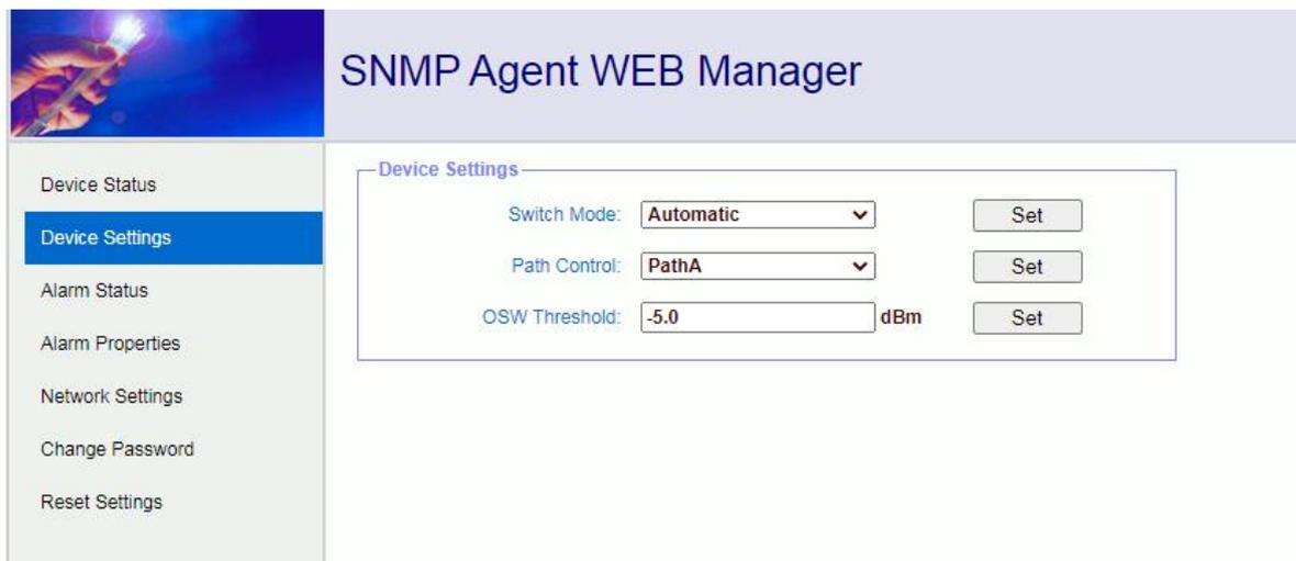
The screenshot shows the 'Device Settings' page of the SNMP Agent WEB Manager. The left sidebar contains navigation options: Device Status, Device Settings (selected), Alarm Status, Alarm Properties, Network Settings, Change Password, and Reset Settings. The main content area displays the following settings:
