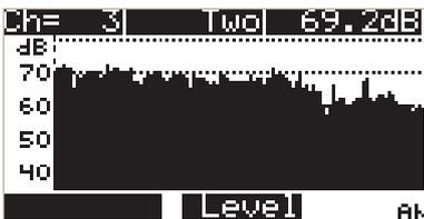
The MSQ-800 can also perform full channel plan scans and Tilt measurements to easily identify problems in the network.
