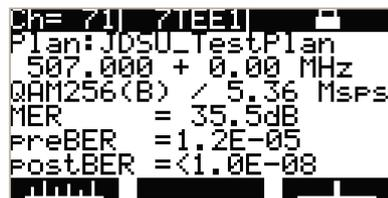
The MSQ-900 performs QAM Annex A/B/C testing on QAM-64/128/256 providing results for MER and Pre/Post-BER measurements.
