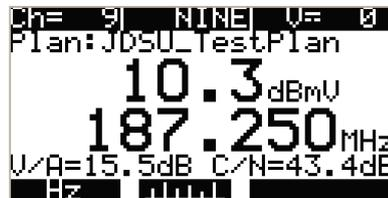
The MSQ-900 performs SLMs on both analog and digital signals.
