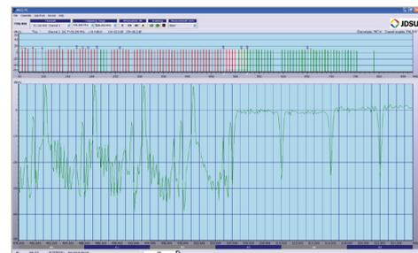
The MSQ-PC main screen shows the Fullscan levels of the active channel plan and individual channel measurements. On the lower panel the MSQ-PC lets users view the downstream spectrum of live RF signals.
