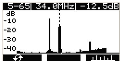
The upstream scan is used to identify ingress in the network.
