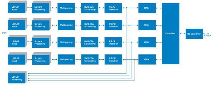
Block Diagram, Quad QAM Out
